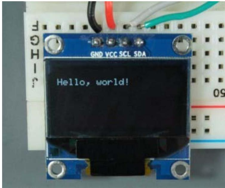
Figure 10: Text message display on OLED
