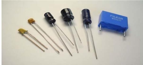
Figure 24: Types of capacitors
