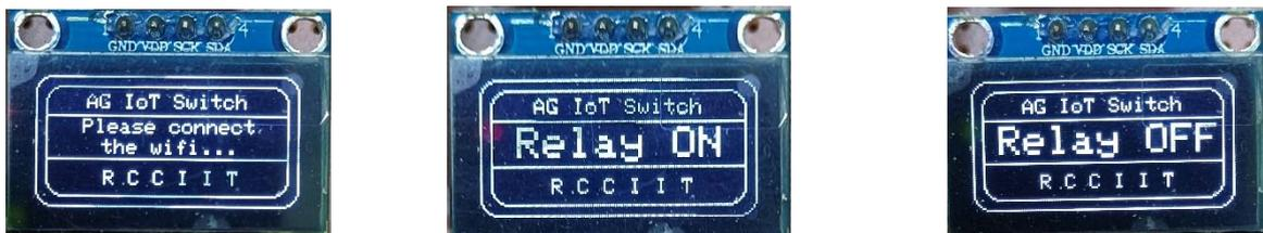
Figure 14: Different messages on the OLED screen
